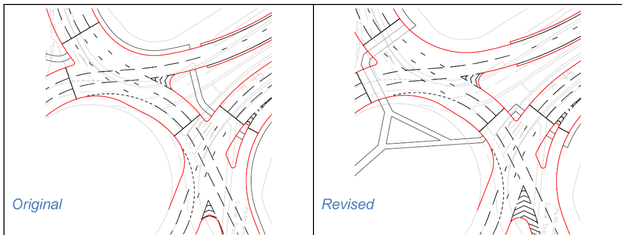
Figure 9 – Comparison of layout options for right turn into cut-through
