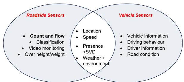
Traffic counting is fundamental to modelling. This work explores the art-of-the-possible for inferring **count and flow** information from vehicle data instead of traditional roadside devices or manual counts. The overlap of vehicle and roadside capability is likely to grow overtime, enabling a potential future where naked roads may also include the reduction and removal of many physical roadside sensors, replaced by methods like we've shown.
