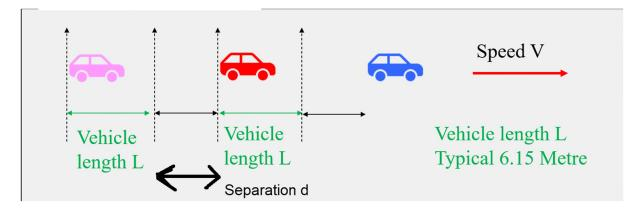
Time between vehicles to passing a fixed point is (L + d) / V secs
