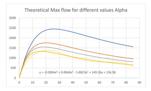
The chart shows flow rate for different speeds (MPH) for values of  $\alpha$  (alpha) being 0.6 (blue), 1 (red), 1.2 (grey) and 1.5 (yellow). The dotted yellow is a 'best fit' quartic curve for the case of  $\alpha$  = 1.5
