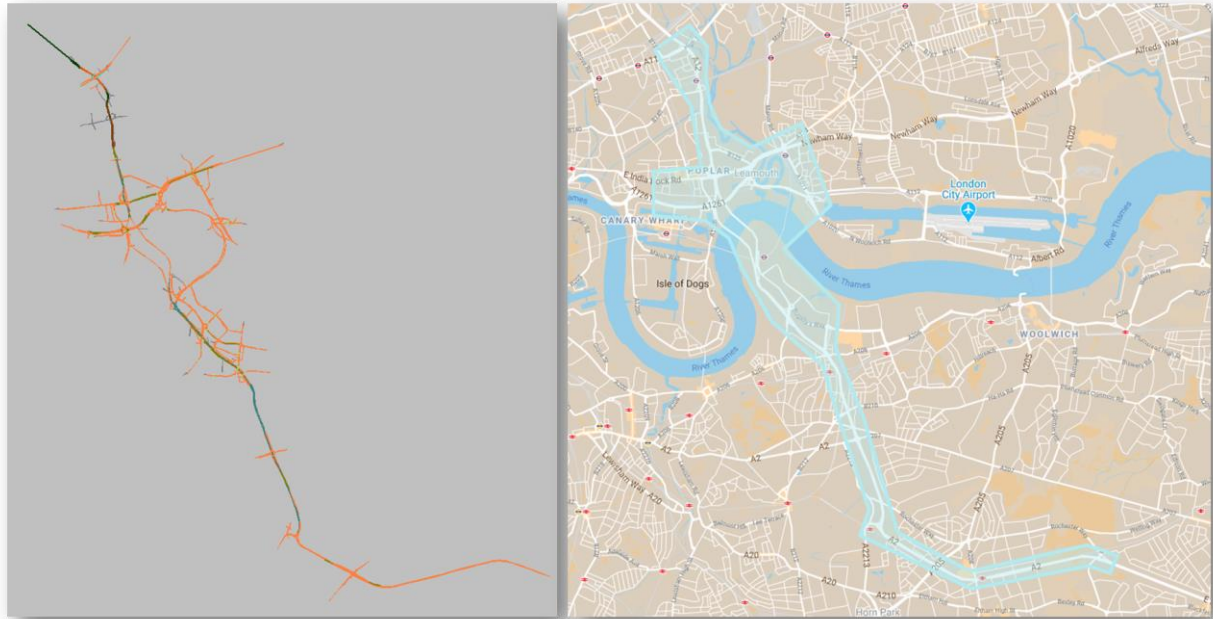
Figure 3: Detail of the VISSIM model used to assess Silvertown Tunnel (left), and the microsimulation study area overlaid on a map (right). The model extended from north of Bow Roundabout to beyond Eltham on the southern side.
